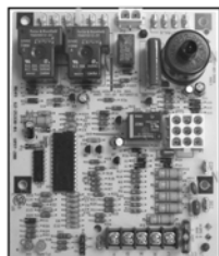
INTEGRATED FURNACE CONTROL
